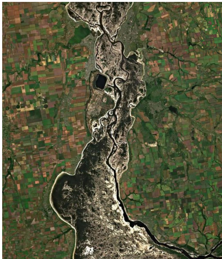
Image 1. Shallowing of the Kakhovka Reservoir after the dam breach in June 2023. Source: Sentinel-2. 17
