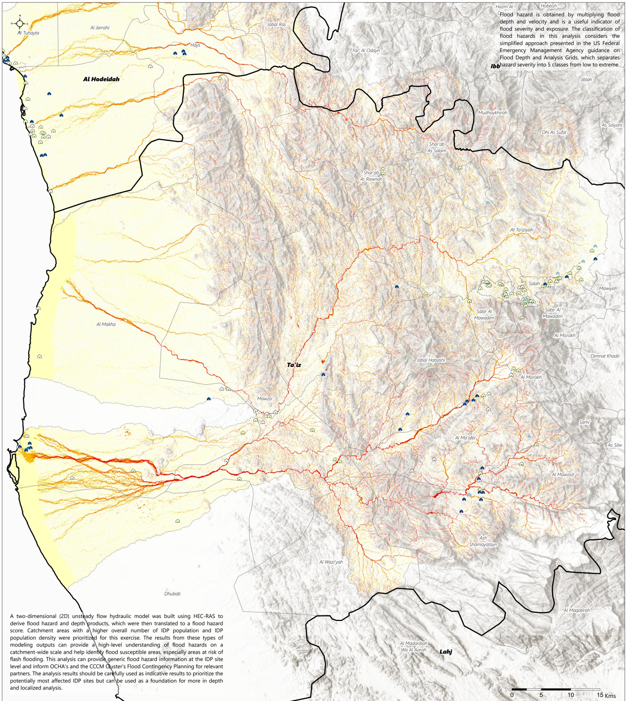
Flood hazard is obtained by multiplying flood depth and velocity and is a useful indicator of flood severity and exposure. The classification of flood hazards in this analysis considers the simplified approach presented in the US Federal Emergency Management Agency guidance on Flood Depth and Analysis Grids, which separates Ibb hazard severity into 5 classes from low to extreme.
