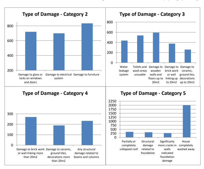
Figure 11: Type of Damage, by Category of Damage
