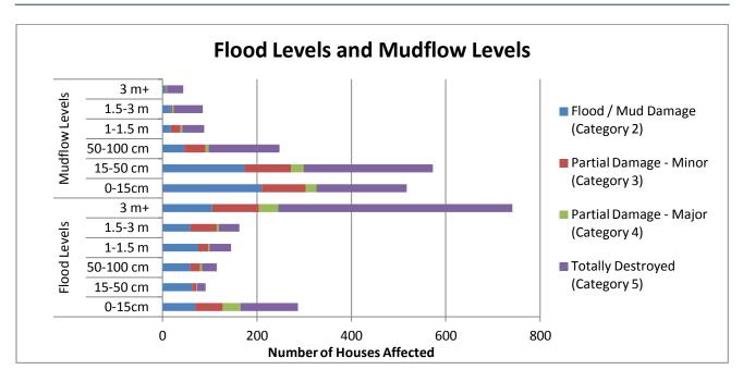
Figure 10: Flood Levels and Mudflow Levels, by Category of Damage
