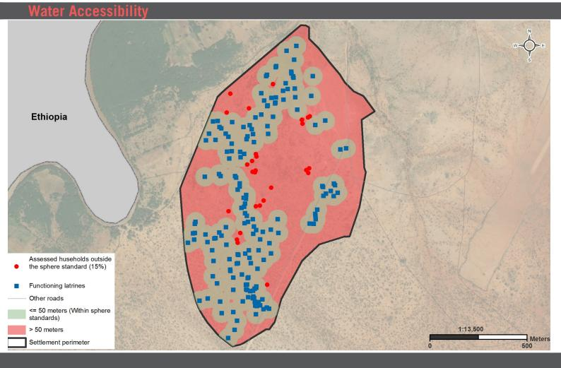
Note Maps: Latrines and water points were mapped during a REACH assessment in April 2017. The number of shelters within and outside a 50m buffer of the latrines was calculated using spatial analysis. The shelters were mapped by UNOSAT using satellite image analysis.
