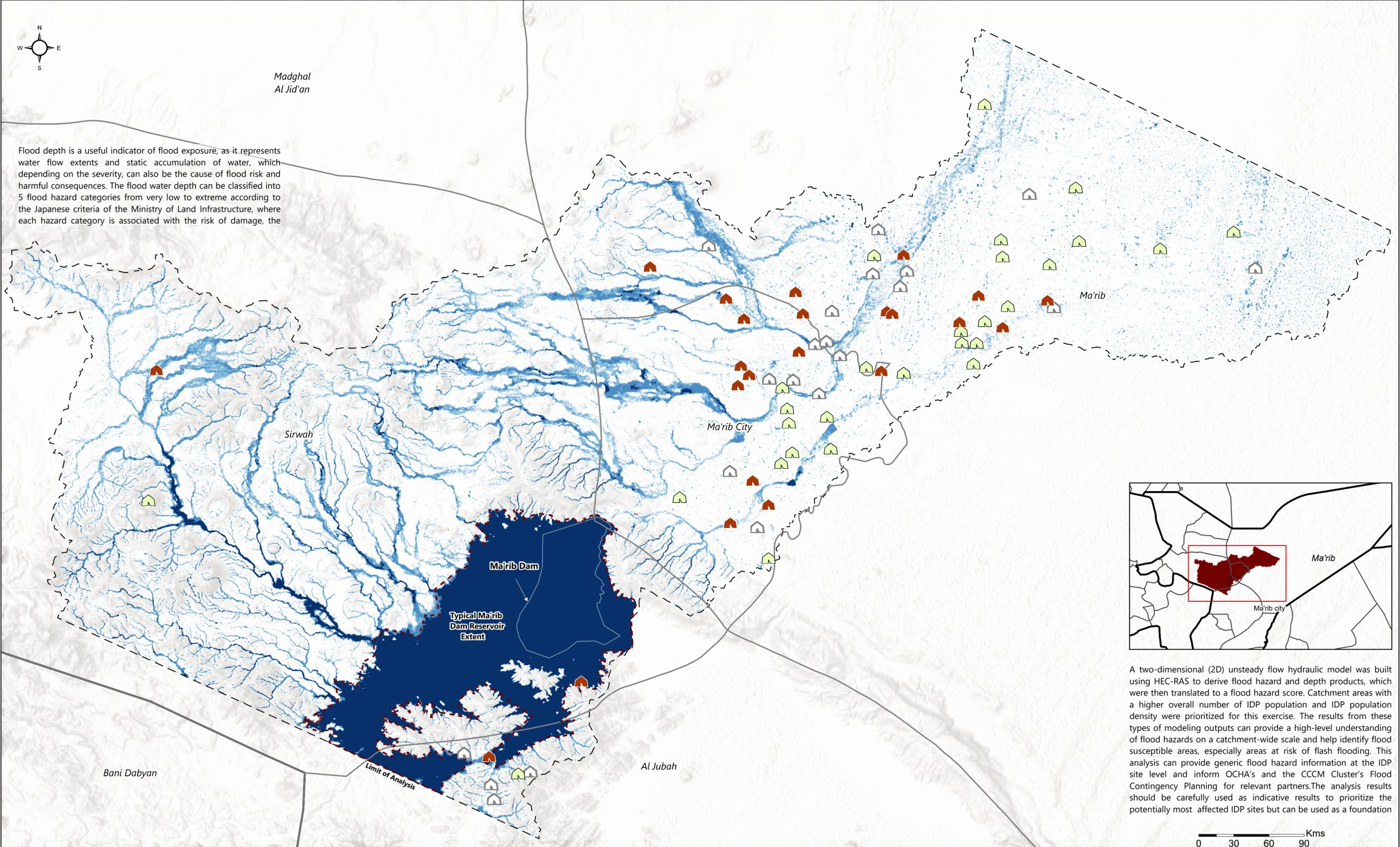
Flood depth is a useful indicator of flood exposure, as it represents water flow extents and static accumulation of water, which depending on the severity, can also be the cause of flood risk and harmful consequences. The flood water depth can be classified into 5 flood hazard categories from very low to extreme according to the Japanese criteria of the Ministry of Land Infrastructure, where each hazard category is associated with the risk of damage, the
