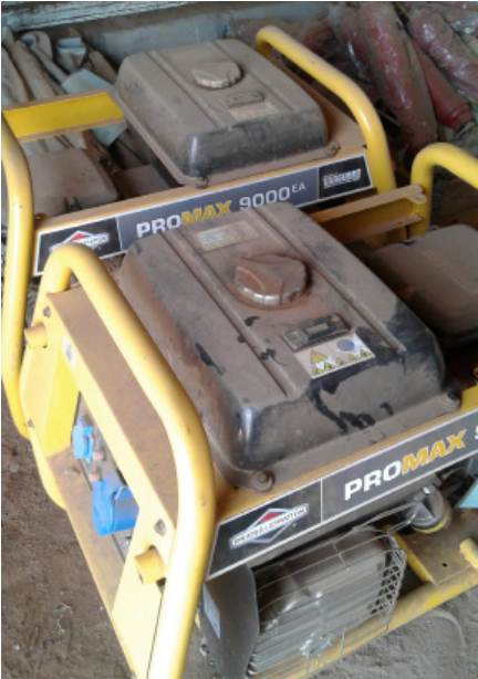
Figure 2: Spare generators for water pump operation in the WASH pipeline warehouse
