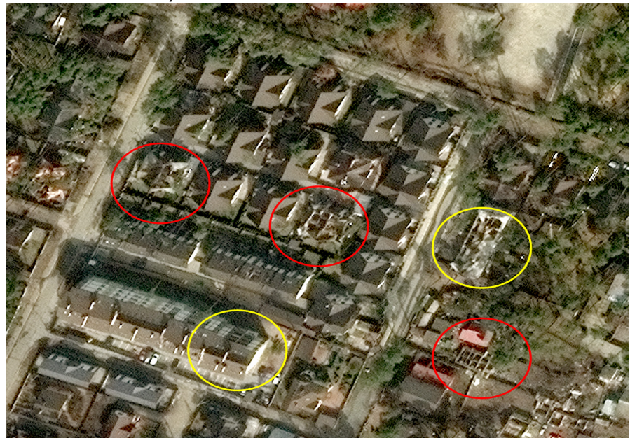
Image 1 and 2: Examples of detected damage to residential buildings in Irpin based on satellite imagery. Red circles - single-household apartments; Yellow circles - apartment buildings; Blue circle - town-house (a group of single-household apartments connected by the common sidewalls).
